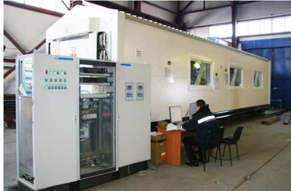
2009 - SIKN for Odoptu-more oilfield, OOO RN-Sakhalinmorneftegas, OAO NK Rosneft. SOI IVK MikroTEK with hot backup
